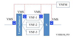
Figure 1 – Example of virtual measurement system (VMS) placement, with management connectivity
