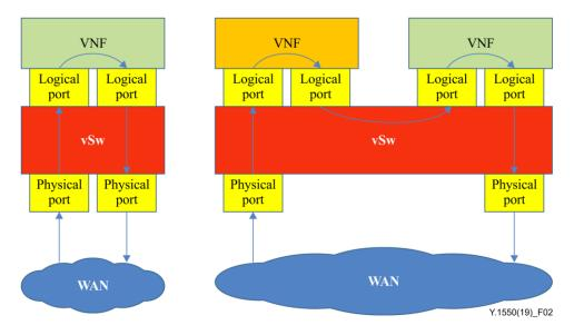
Figure 2 – Example of virtual measurement system (VMS) deployment on the service path
