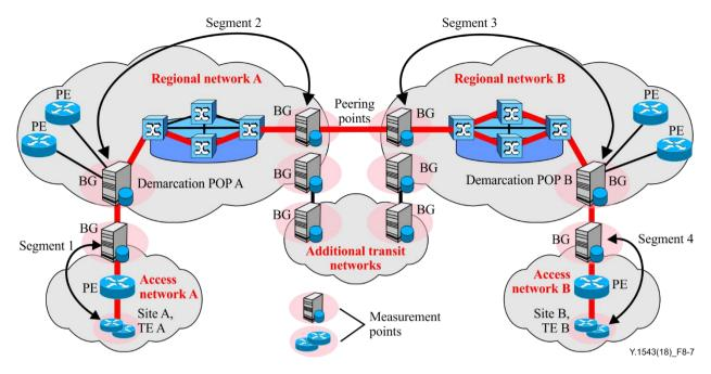
Figure 8-7 – Passive measurement based on the real-time transport protocol/real-time transport control protocol
