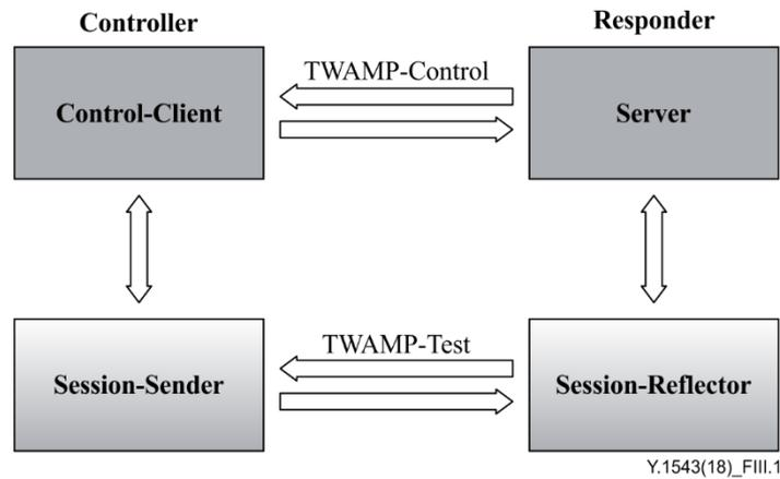
**Figure III.1 – Two-way active measurement protocol architecture**
