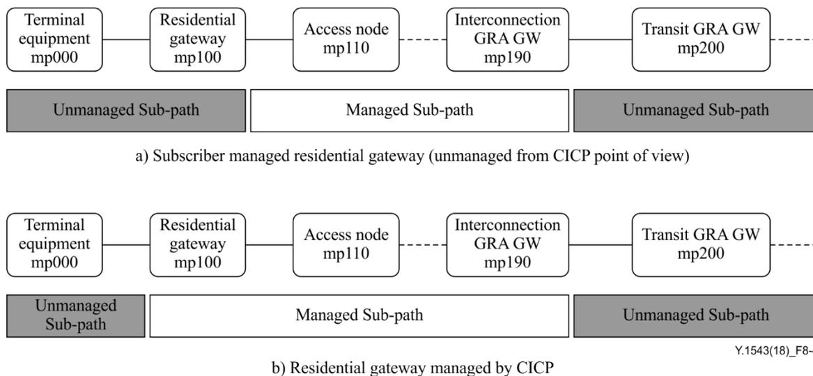
**Figure 8-4 – TE-CE-PE model (TE=mp000, CE=mp100, Ingress PE=mp110)**
