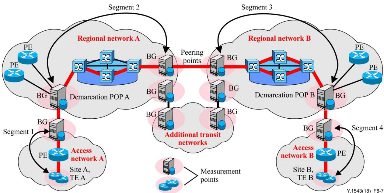
**Figure 8-7 – Passive measurement based on the real-time transport protocol/real-time transport control protocol**
