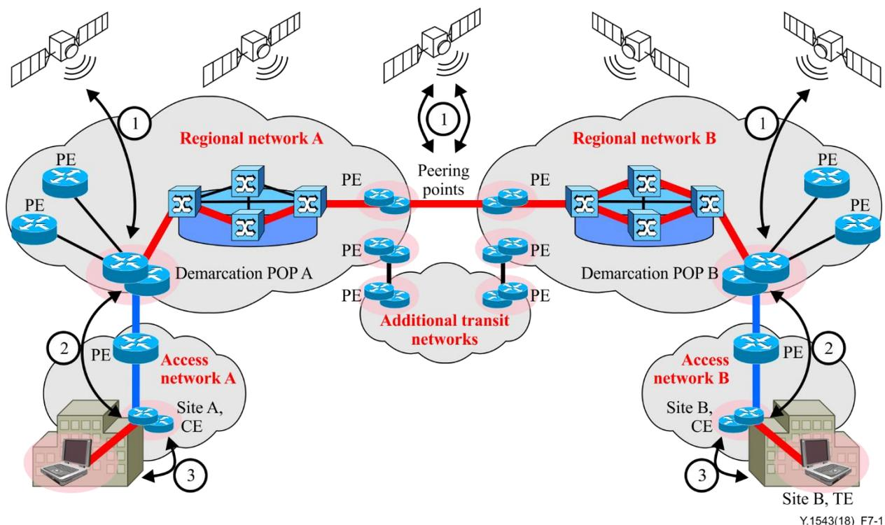
**Figure 7-1 – Three categories of equipment at which offset maxima apply**
