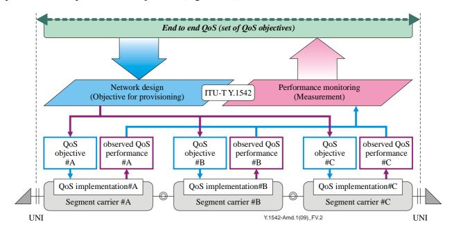
Figure V.2 – End-to-end QoS performance objectives and multi-domain network
