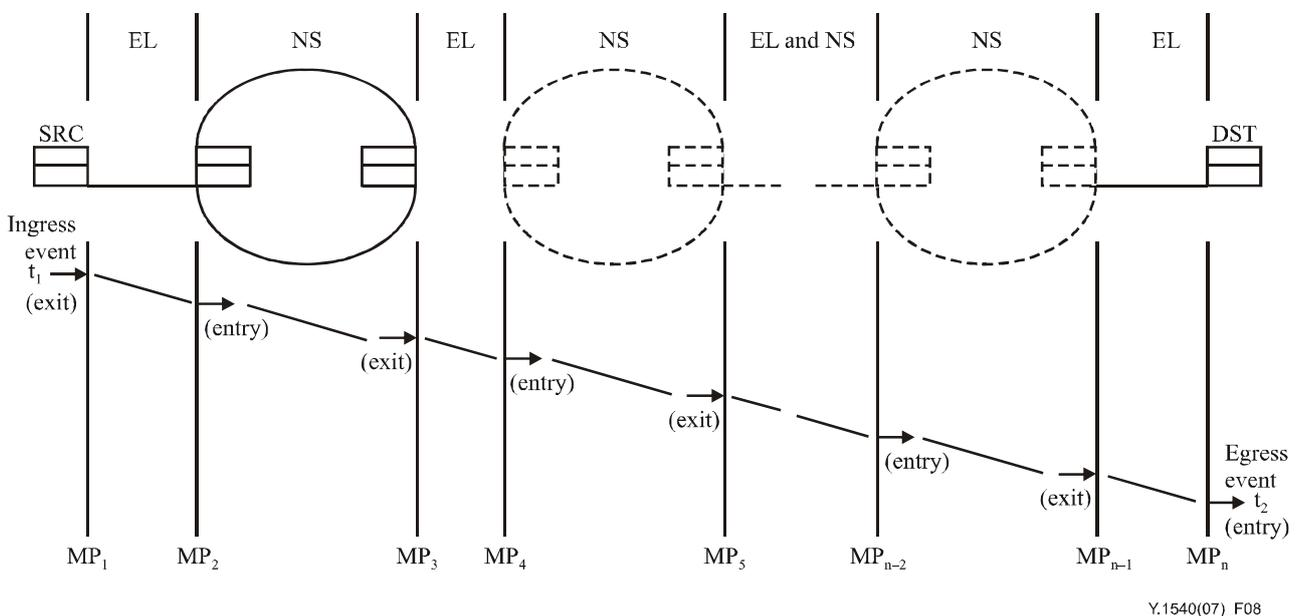
**Figure 8 – IP packet transfer delay events**
