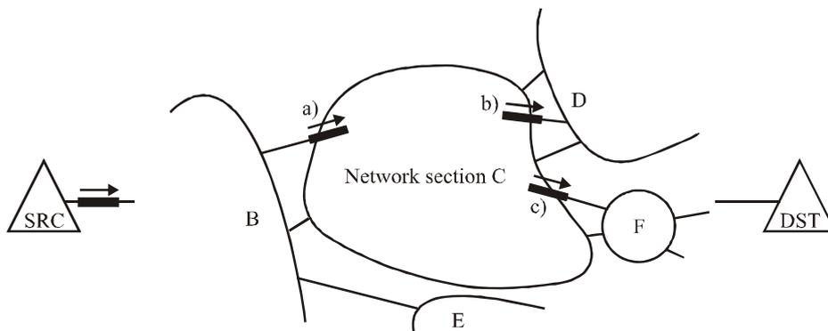
An IP packet from SRC to DST enters NS C, creates an ingress event, is fragmented, and creates two corresponding egress events, b) and c).
