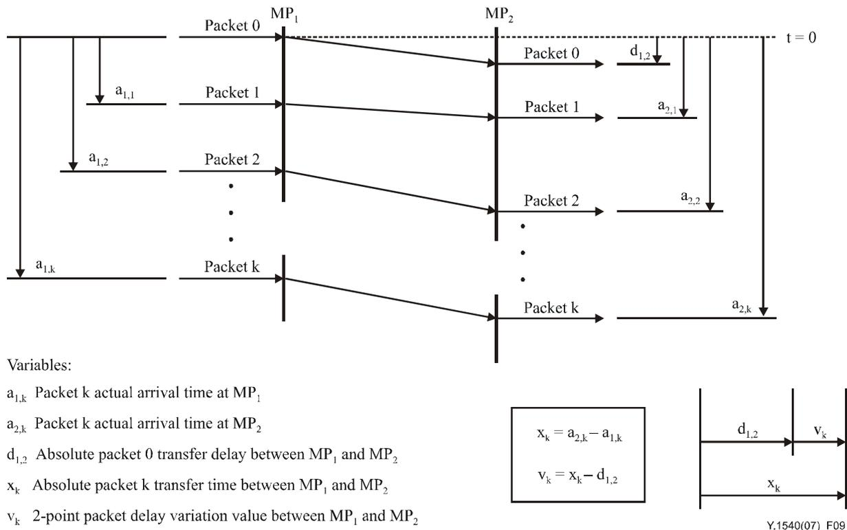
**Figure 9 – 2-point IP packet delay variation**
