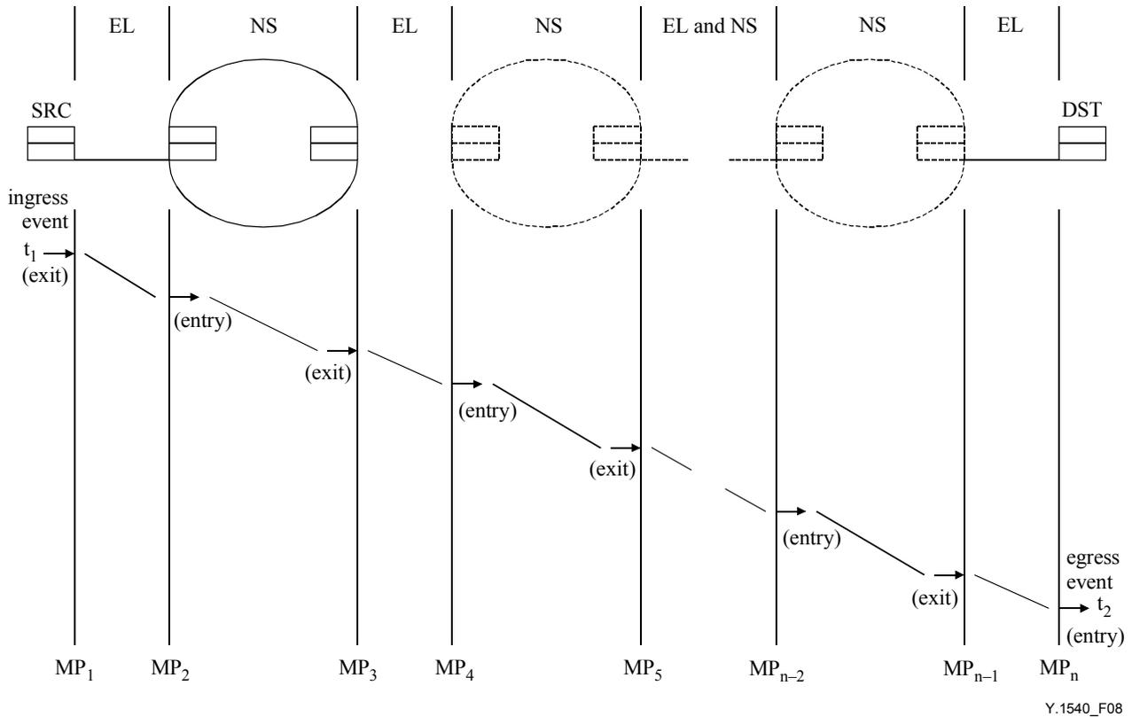
**Figure 8/Y.1540 – IP packet transfer delay events
