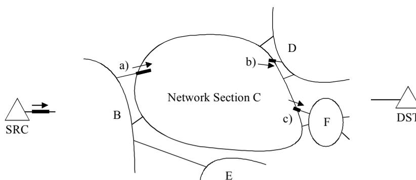
An IP packet from SRC to DST enters NS C, creates an ingress event, is fragmented, and creates two corresponding egress events, b) and c).
