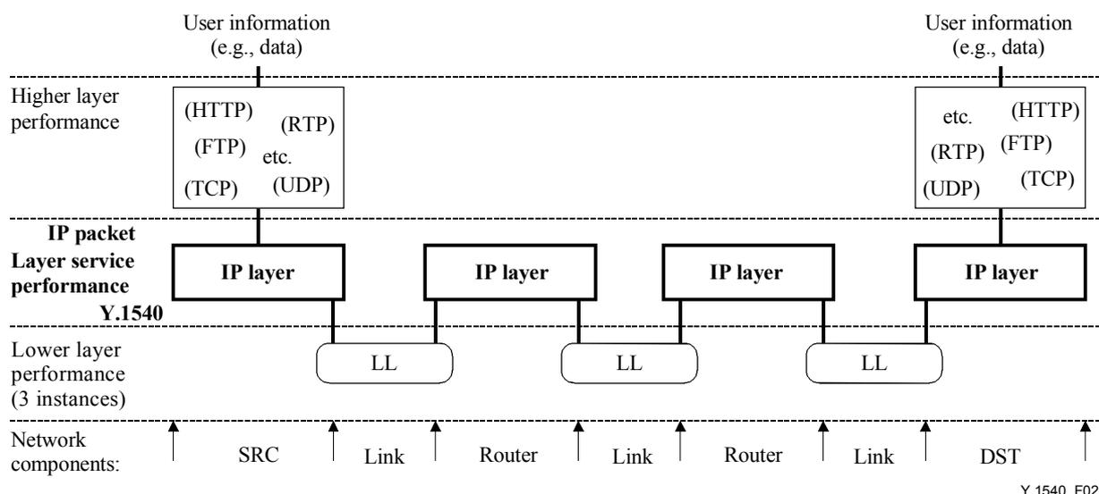
**Figure 2/Y.1540 – Layered model of performance for IP service – Example**
