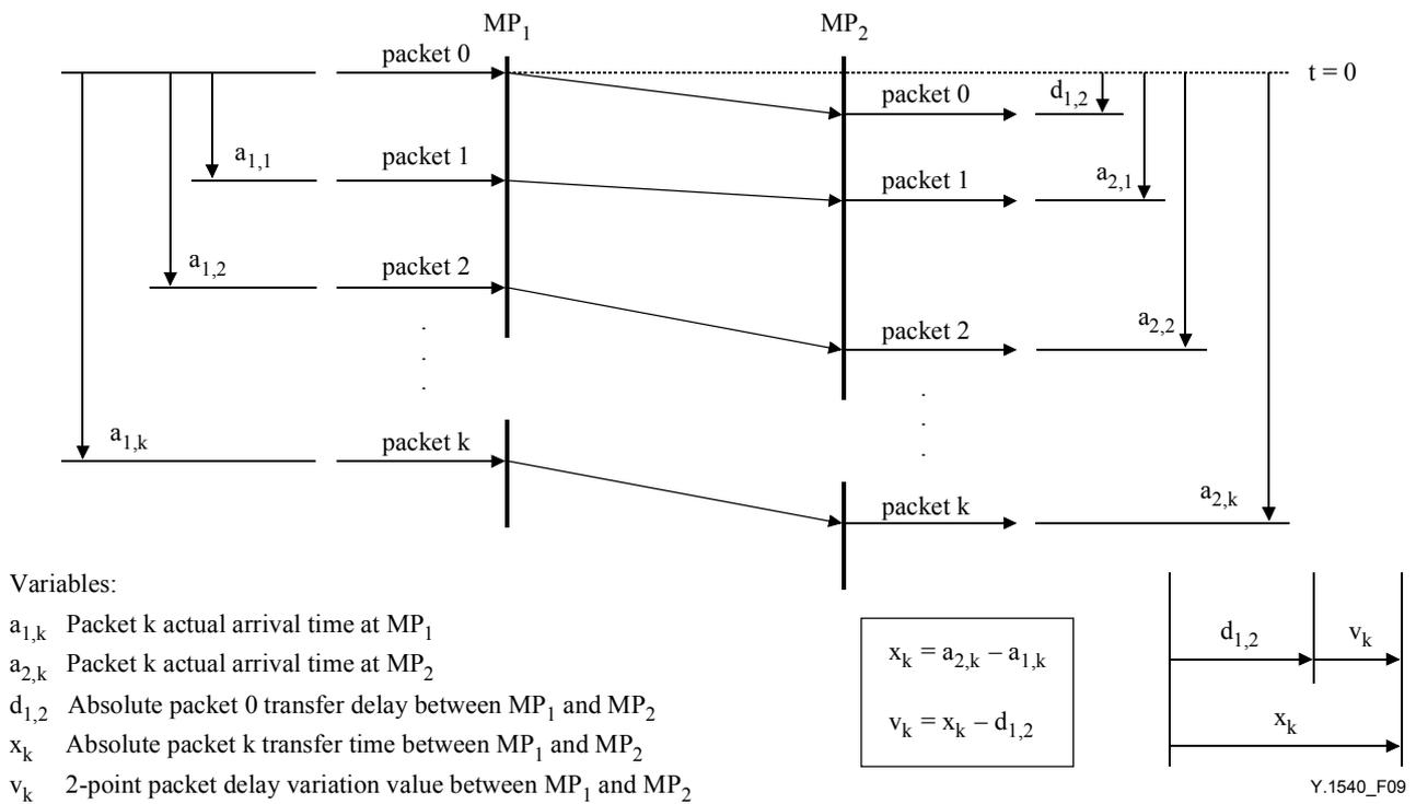
**Figure 9/Y.1540 – 2-point IP packet delay variation**
