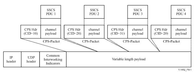
Figure 9-1/Y.1452 – Packing of CPS packets into an IP packet
