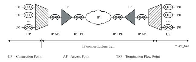
Figure 6-2/Y.1452 – Functional architecture for multiplexing P0 channels over IP networks
