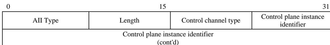
**Figure 2 – SAI and TAI format for control PW setup**
