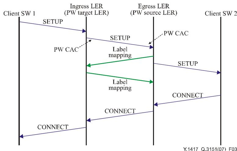
**Figure 3 – PW establishment triggered by client connection SETUP at egress LSR**
