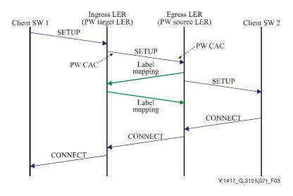
Figure 3 – PW establishment triggered by client connection SETUP at egress LSR
