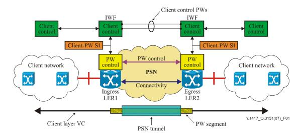
Figure 1 – High-level architecture
