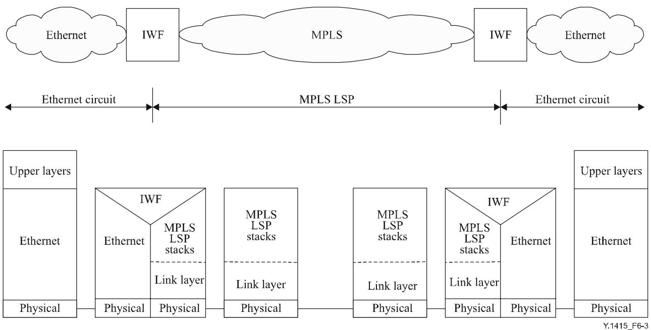
**Figure 6-3/Y.1415 – Network reference model and protocol layers for Ethernet-MPLS user plane interworking**
