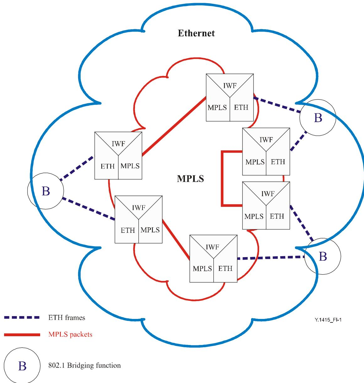
**Figure I.1/Y.1415 – Ethernet network with multipoint connectivity supported by Interworking LSPs**
