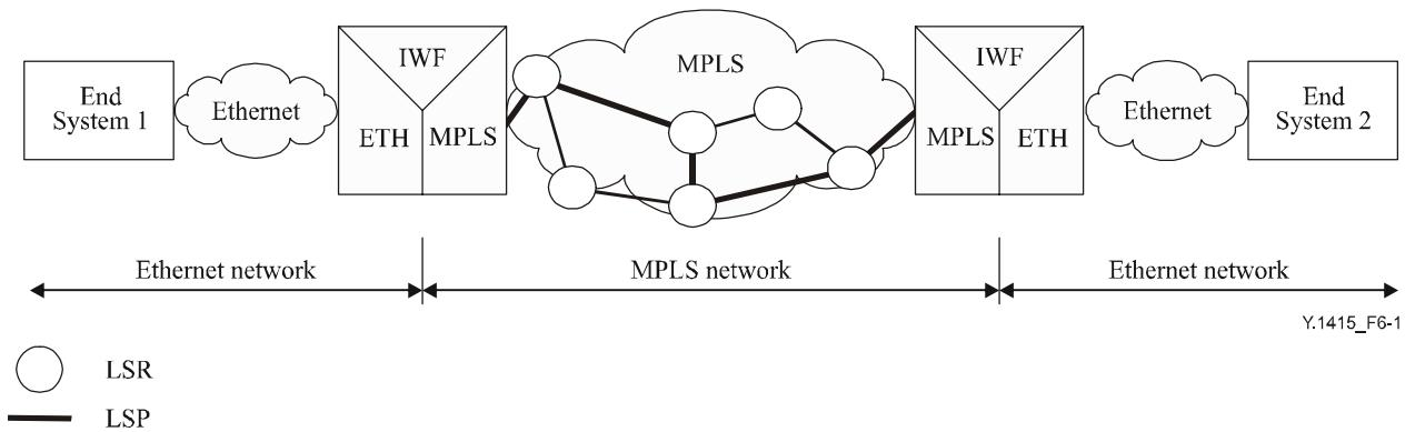
**Figure 6-1/Y.1415 – Reference architecture for Ethernet-MPLS network interworking**
