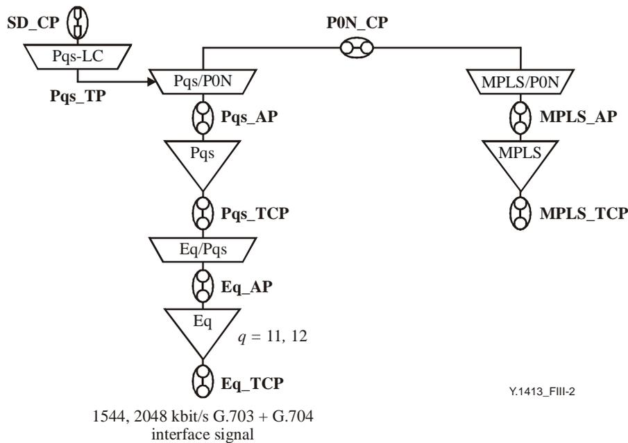
NOTE – P0N represents the  $n \times 64$  kbit/s signal (with or without CAS/CCS).
