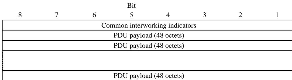
**Figure 9-5/Y.1413 – Structure-indicated encapsulation with multiple PDUs per packet**
