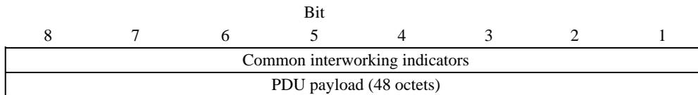
**Figure 9-4/Y.1413 – Structure-indicated encapsulation with a single PDU per packet**
