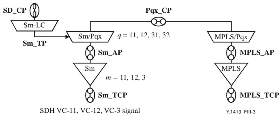
**Figure III.3/Y.1413 – Structure-agnostic TDM over MPLS functional model for 1544, 2048, 34368 and 44736 kbit/s PDH signals carried over SDH VC-m**
