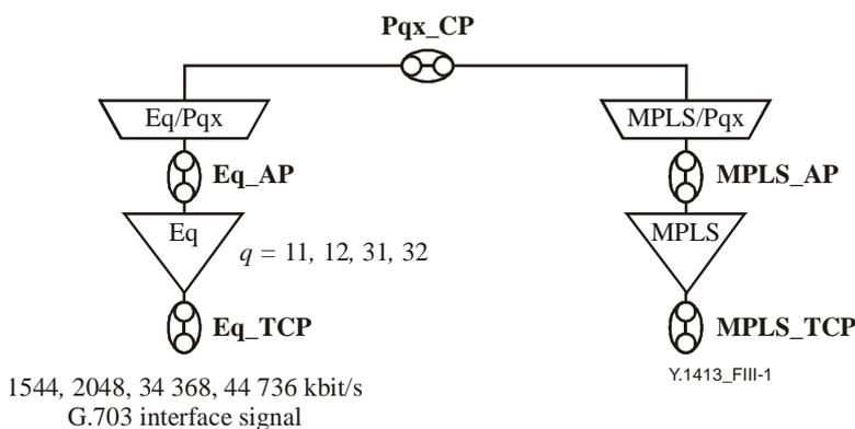
**Figure III.1/Y.1413 – Structure-agnostic TDM over MPLS functional model for 1544, 2048, 34 368 and 44 736 kbit/s PDH signals**
