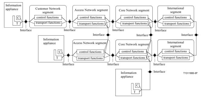
Figure 2/Y.130 – An example of horizontal network components (extracted from ITU-T Recommendation Y.110)
