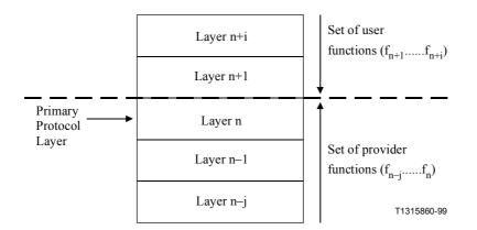
Figure 6/Y.130 – Generic layered protocol stack architecture
