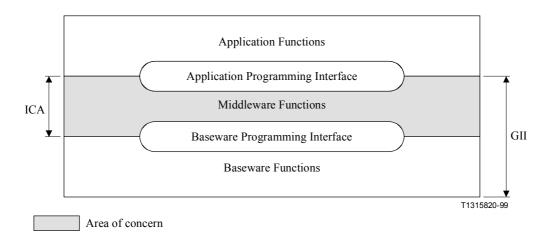
Figure 1/Y.130 – Vertical scope and relationship between the ICA and the GII
