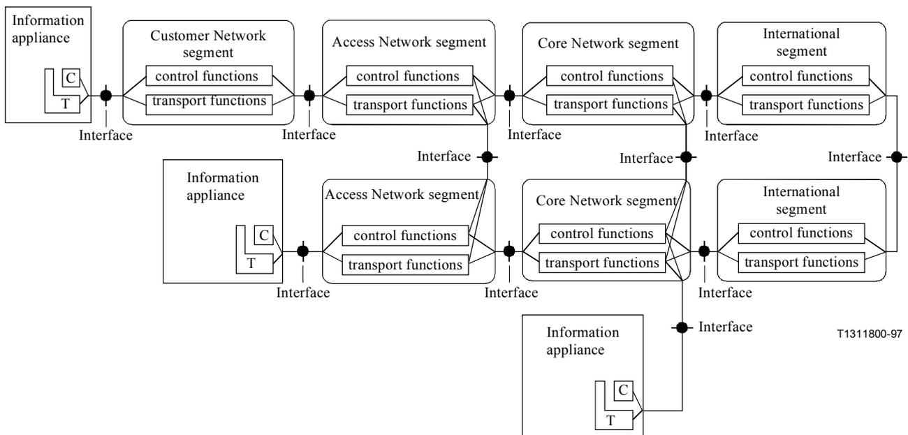
**Figure 2/Y.130 – An example of horizontal network components
