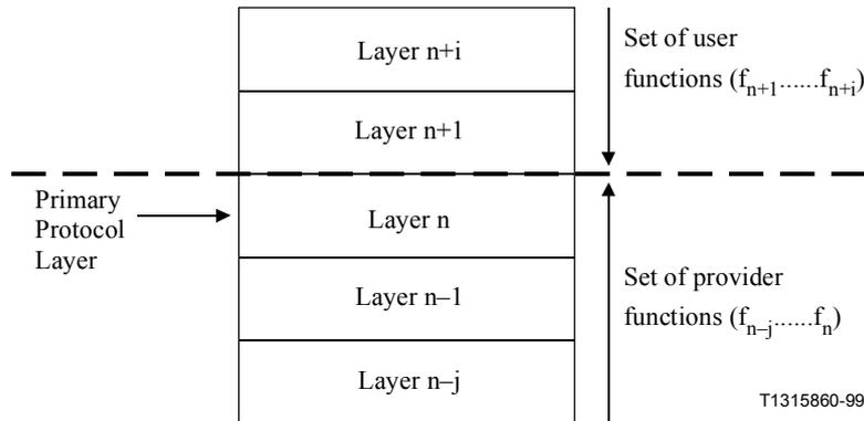
**Figure 6/Y.130 – Generic layered protocol stack architecture**
