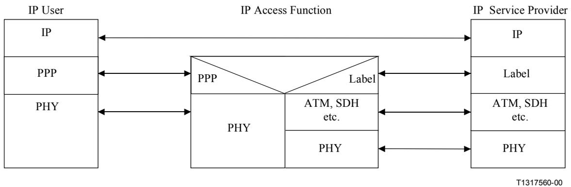
**Figure 9/Y.1231 – Functional model of MPLS**
