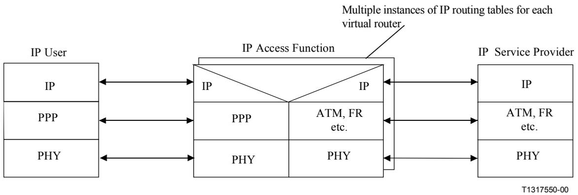
**Figure 8/Y.1231 – Functional model of virtual router**
