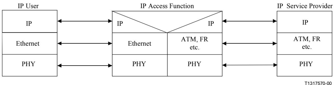
**Figure 10/Y.1231 – Functional model of Ethernet use**
