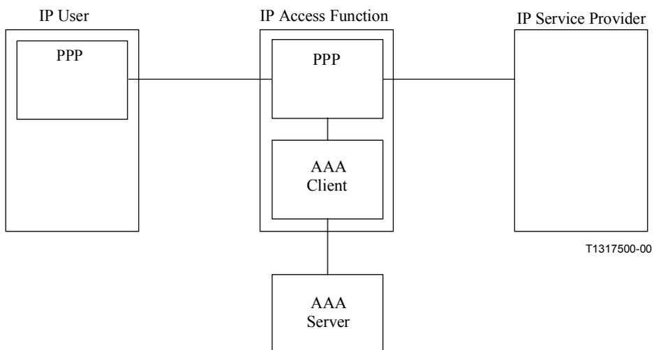
**Figure 3b/Y.1231 – PPP terminated aggregation**
