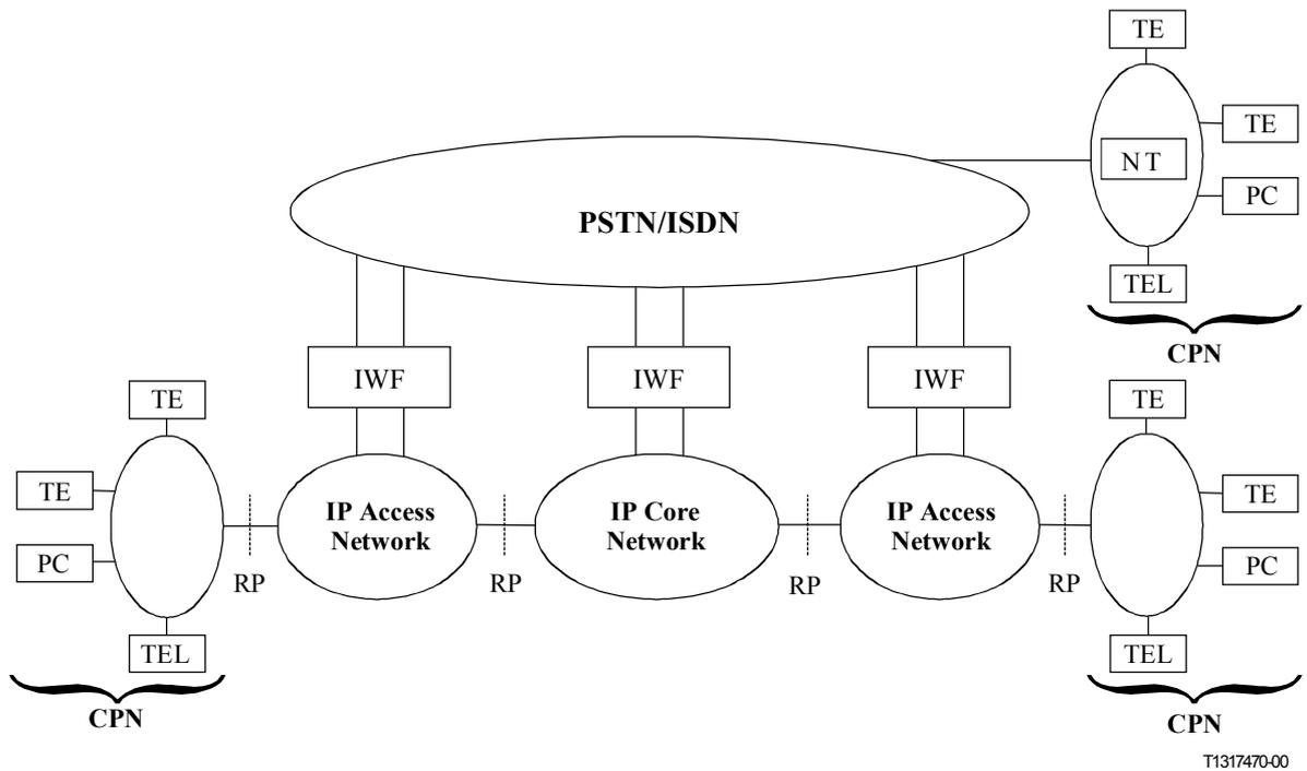
**Figure 1b/Y.1231 – An example of relationship between IP network and PSTN/ISDN**
