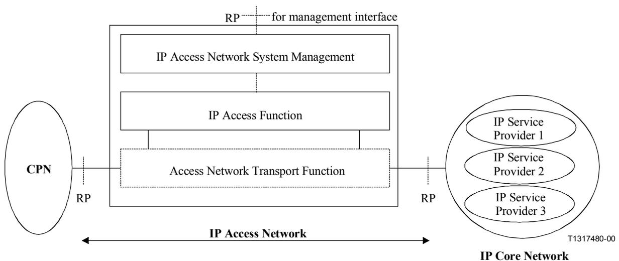
**Figure 2/Y.1231 – IP Access Network architecture example**
