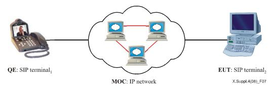
Figure 7 – Example of the basic interoperability test architecture for SIP phones
