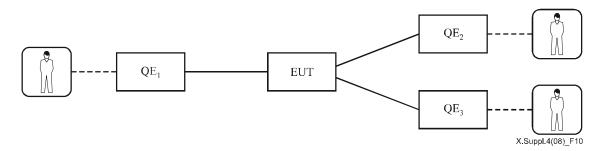
Figure 10 – Basic interoperability architecture with three QEs and no EUT test driver
