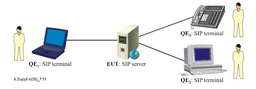
Figure 11 – Using three QEs to test the call diversion service
