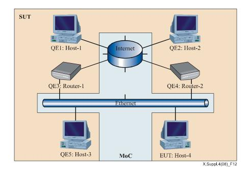
Figure 12 – Interoperability testing of an IP host with multiple QEs
