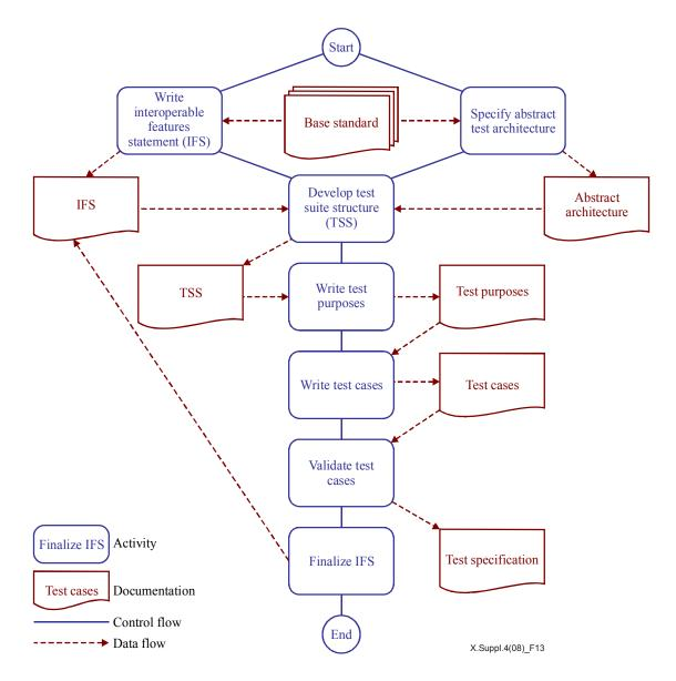
Figure 13 – Developing an interoperability test specification
