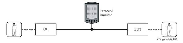
Figure 3 – Interoperability testing with conformance monitoring
