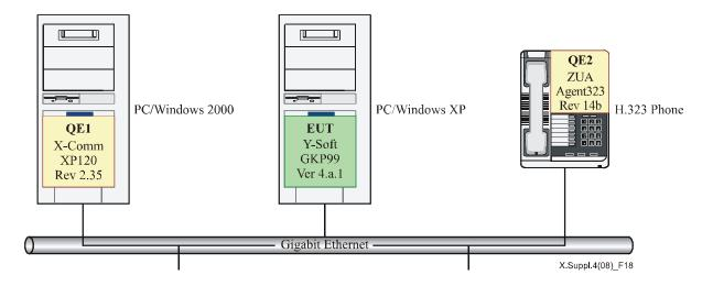
Figure 18 – Test arrangement based on the example abstract architecture
