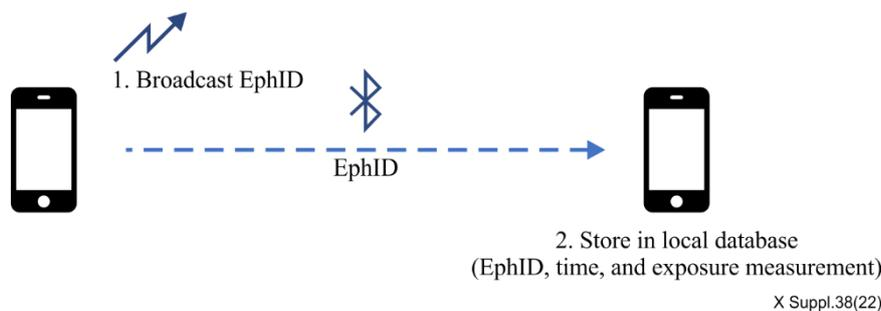
Figure I.1 – Generation and storage of ephemeral IDs (Redrawn from [b-DP<sup>3</sup>T])
