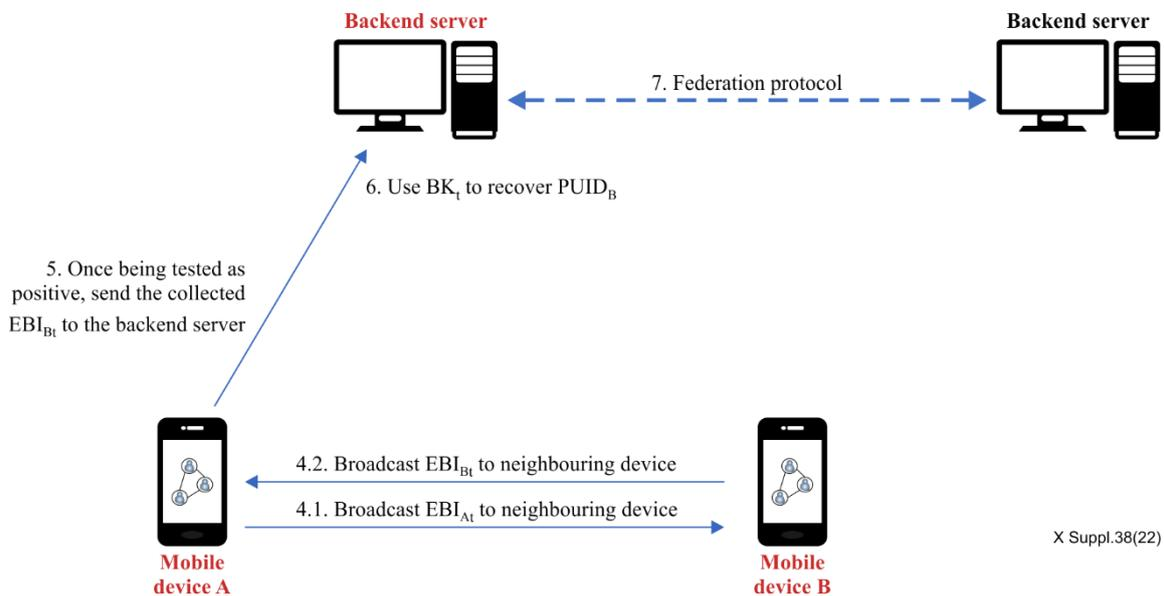
**Figure I.4 – Sharing proximity data with the backend server and federation with other backend server (redrawn from [b-PEPP-PT])**
