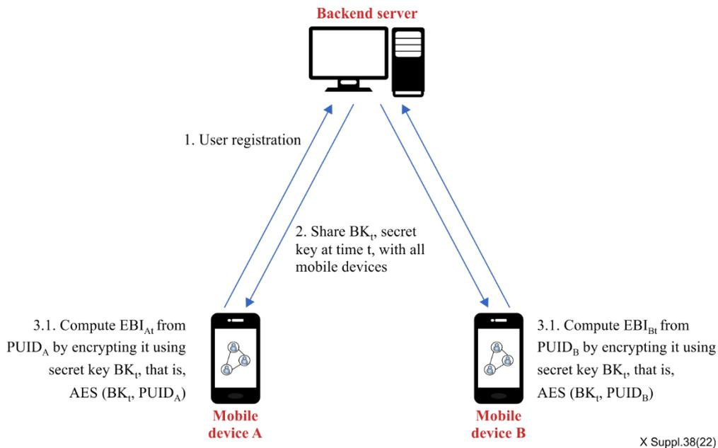
**Figure I.3 – User registration and generation and storage of the encrypted pseudonymous persistent user ID (PUID) and encrypted PUID  $EBI_t$  (Redrawn from [b-PEPP-PT])**
