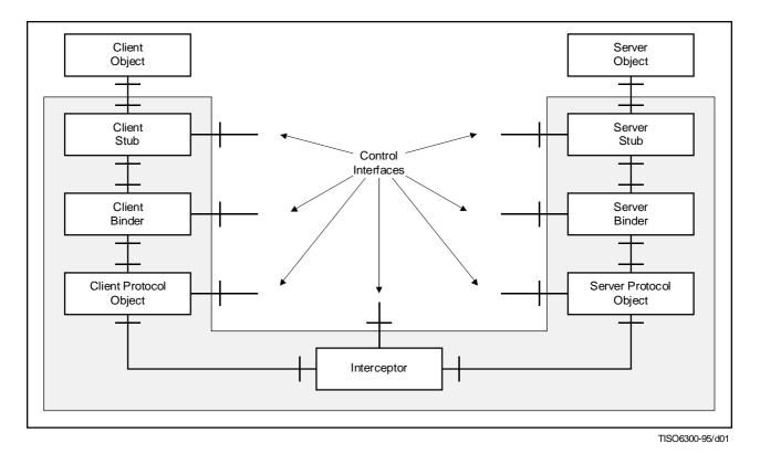
Figure 2 – An example of a basic client/server channel
