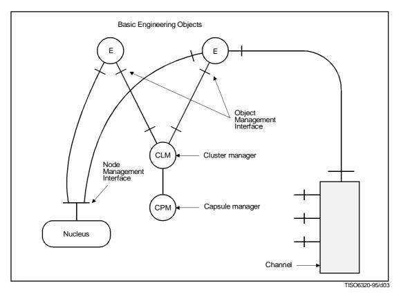
Figure 4 – Example structure supporting a basic engineering object
