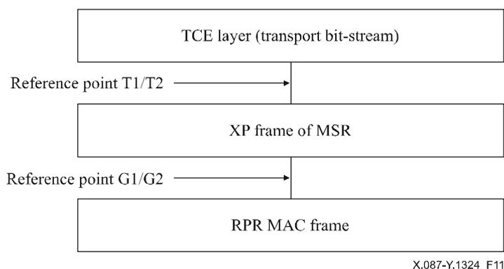
**Figure 11/X.87/Y.1324 – TDM service channel over MSR**
