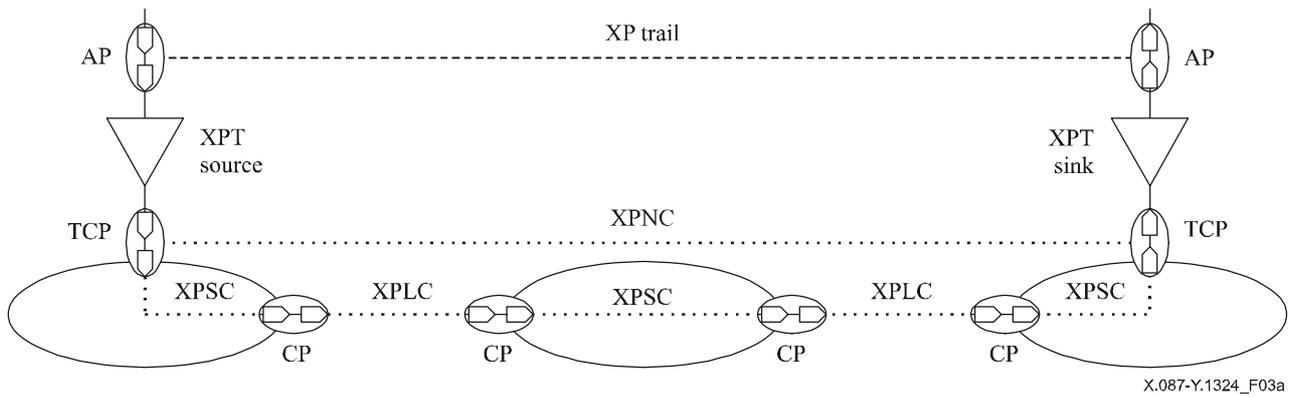
**Figure 3a/X.87/Y.1324 – XP layer network example**
