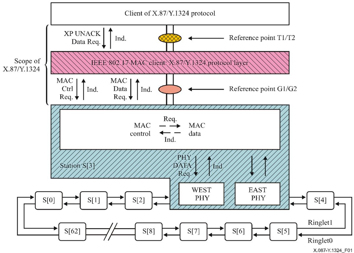
**Figure 1/X.87/Y.1324 – Scope of X.87/Y.1324 based on RPR as a MAC client**
