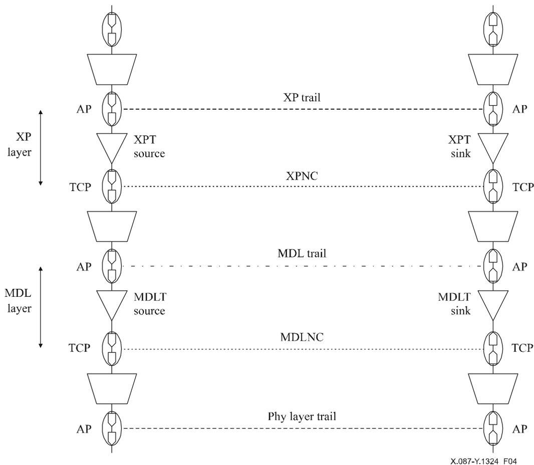
**Figure 4/X.87/Y.1324 – Client/server association in a MSR transport ring**
