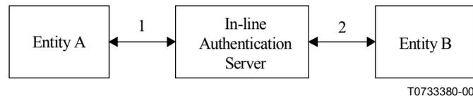
**Figure 9 – Example for In-line TTP Authentication Service**
