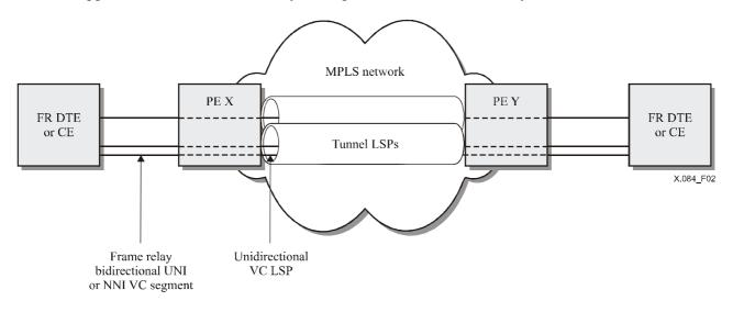
Figure 2/X.84 – Tunnel and VC LSPs
