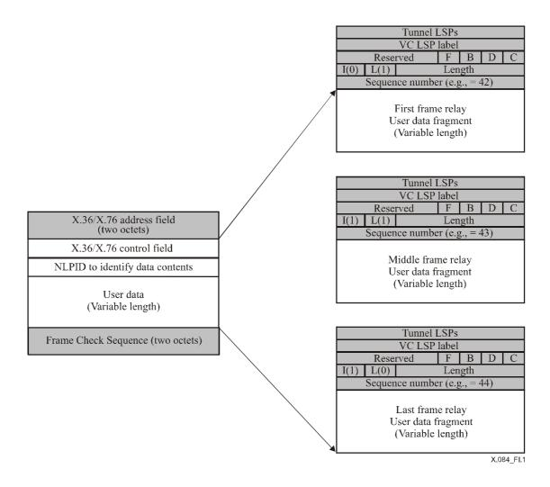
Figure I.1/X.84 – Example of fragmentation for the one-to-one mapping mode
