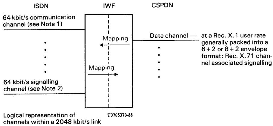
*Note 1* – 64 kbit/s communication channel bearing a data channel at a Rec. X.1 user rate (non-transparent ISDN connection).
