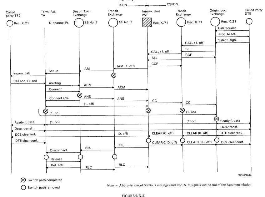
Signalling conversion of a basic call from
