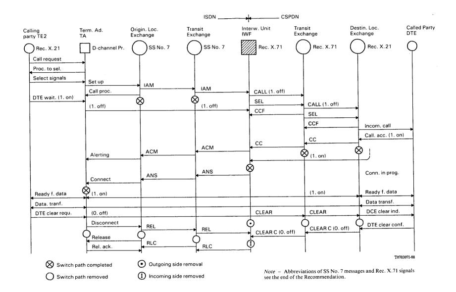
Signalling conversion of a basic call from ISDN to CSPDN
