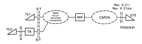
Note - In cases where a TE1-type terminal is used, the bit stream at the S/T-interface complies with the Rec. X.30 frame structure.
