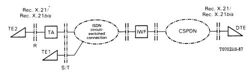
TE1ISDN Terminal Equipment Type 1 (Note)TE2ISDN Terminal Equipment Type 2TE2 and DTEBelonging to the same user class (in user classes of service 3-7)
