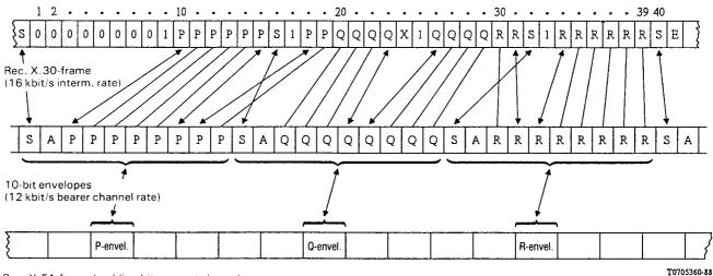
Rec. X.51-frame (padding bits are not shown) (64 kbit/s multiplexed bit stream)
