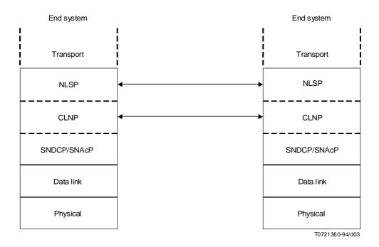
Figure 4 – Illustration of NLSP-CL between end systems
