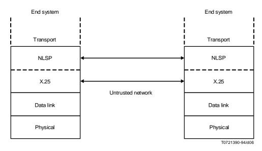
Figure 7 – Illustration of NLSP-CO between end systems
