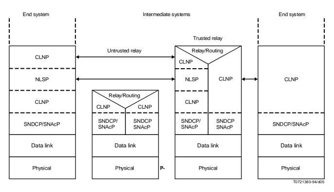
Figure 6 - Illustration of NLSP-CL with untrusted relay system
