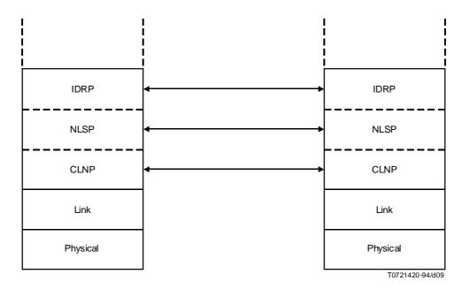
Figure 10 – Illustration of NLSP operating in conjunction with IDRP
