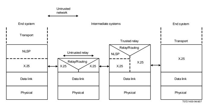
Figure 8 - Illustration of NLSP-CO with untrusted relay system
