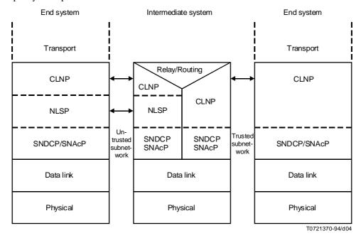
Figure 5 – Illustration of NLSP-CL with untrusted subnetwork
