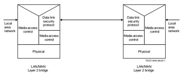
Figure 12 – Illustration of data link layer security protocol used to protect communication between two bridges
