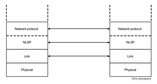
Figure 11 – Illustration of NLSP operating over link layer
