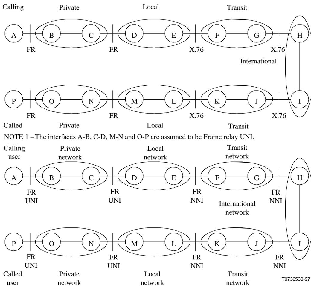
**Figure B.1/X.76 – Reference configuration for location field generation**
