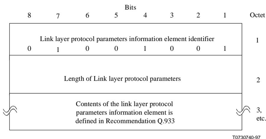
**Figure 10-22/X.76 – Link layer protocol parameters information element**
