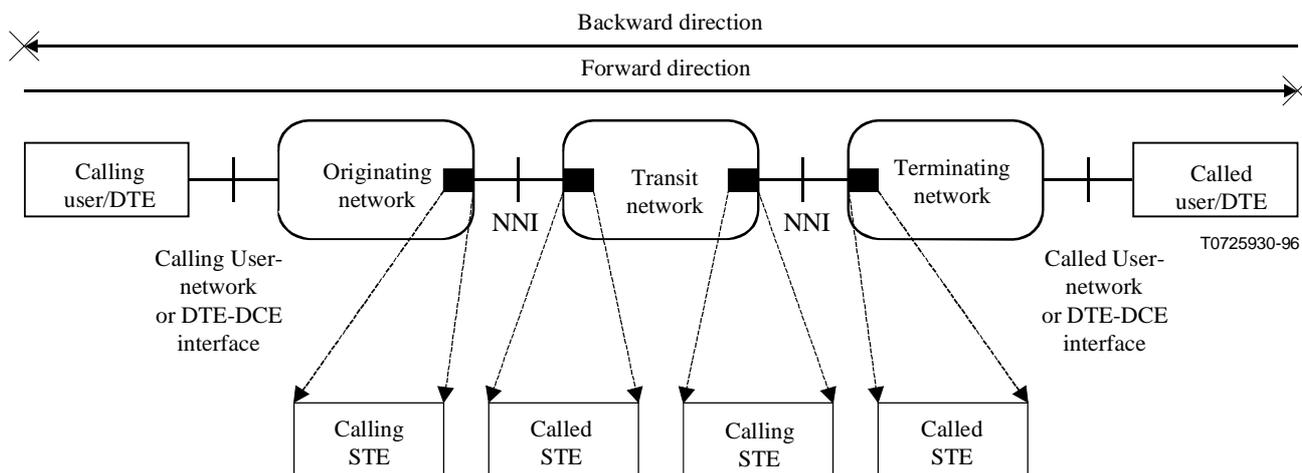
**Figure 10-1/X.76 – Convention used for SVC signalling**
