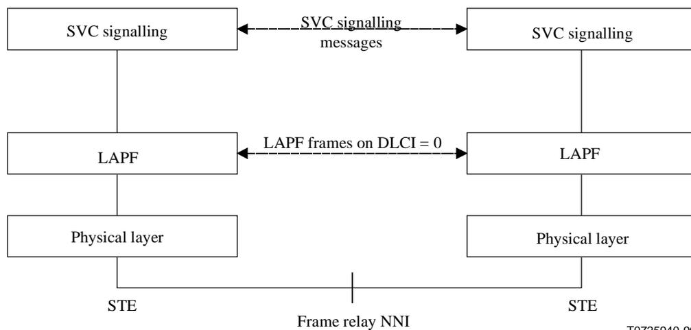
**Figure 10-2/X.76 – STE/STE protocol layers for signalling**
