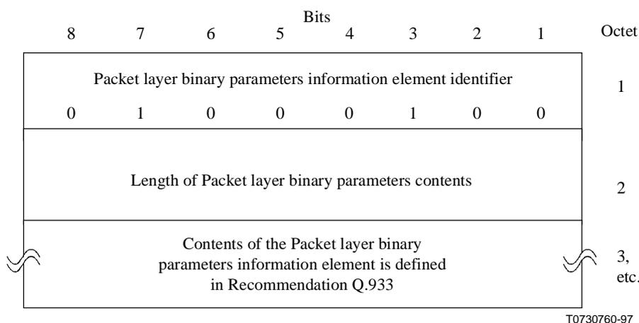
**Figure 10-24/X.76 – Packet layer binary parameters information element**
