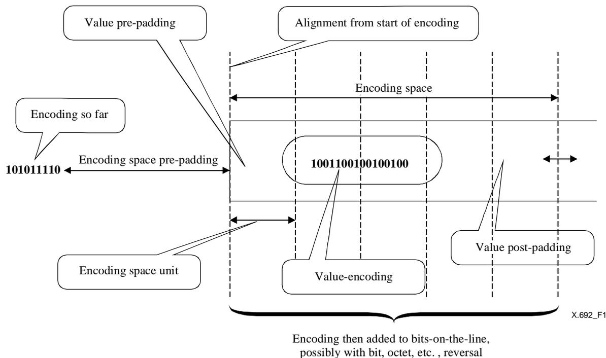
**Figure 1 – Encoding space, value-encoding and padding concepts**
