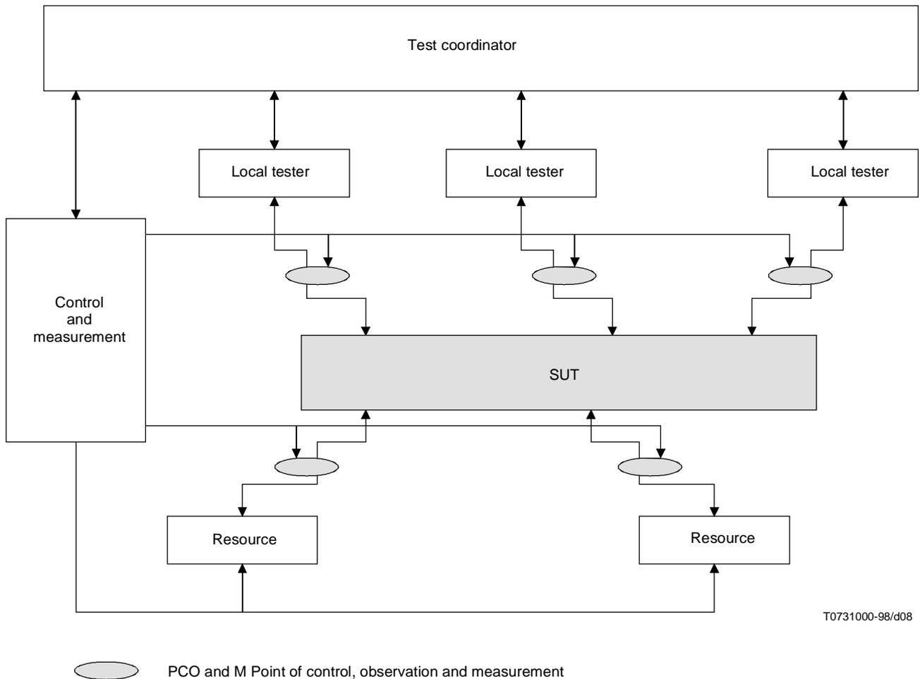
Figure 9-2 – QoS-based service testing architecture
