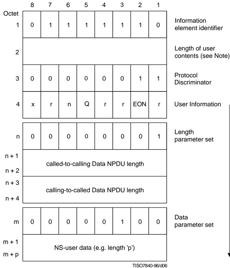
NOTE – The Length of the user contents field is a binary value where bit 1 is the low order bit. The value of the field is determined as follows.
