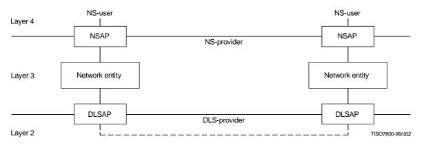
Figure 1 – Model of the network layer
