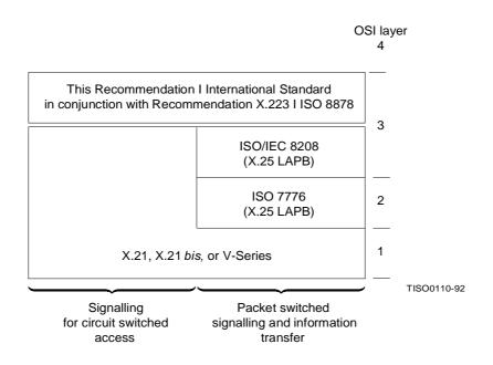
Figure 4 – Protocol layers at R reference point
