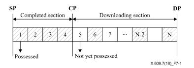
Figure 7-1 – Structure of buffer
