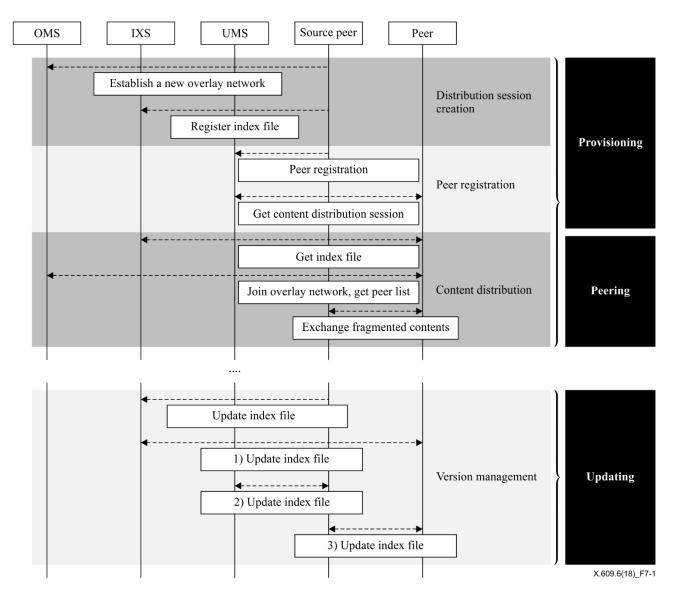
**Figure 7-1** – **High-level procedures for content distribution service**
