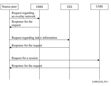
Figure A.1 – Source-side procedure of content distribution
