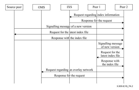
**Figure A.2 – Peer-side procedure of content distribution**
