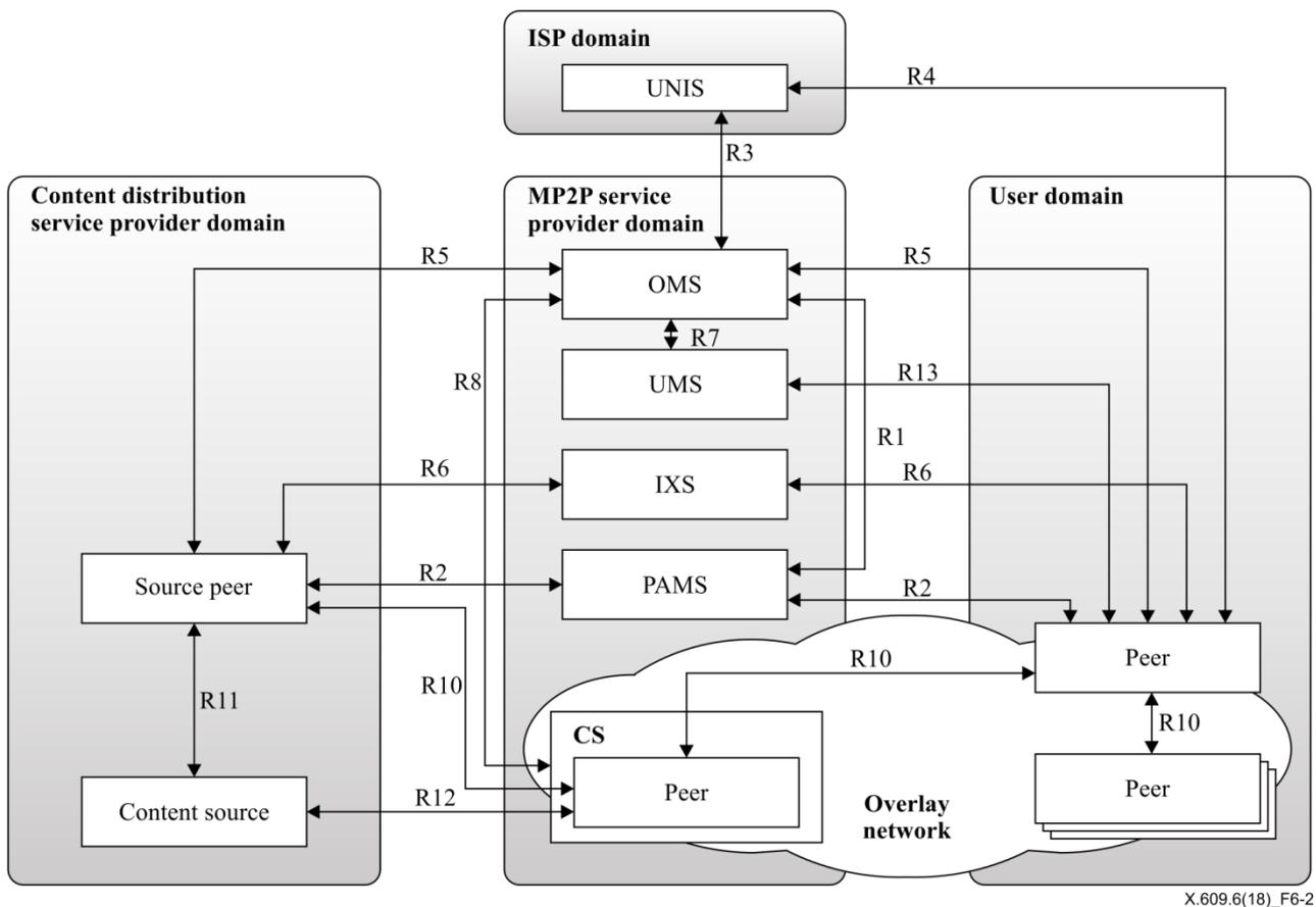
**Figure 6-2 – Extended MP2P architecture for content distribution**
