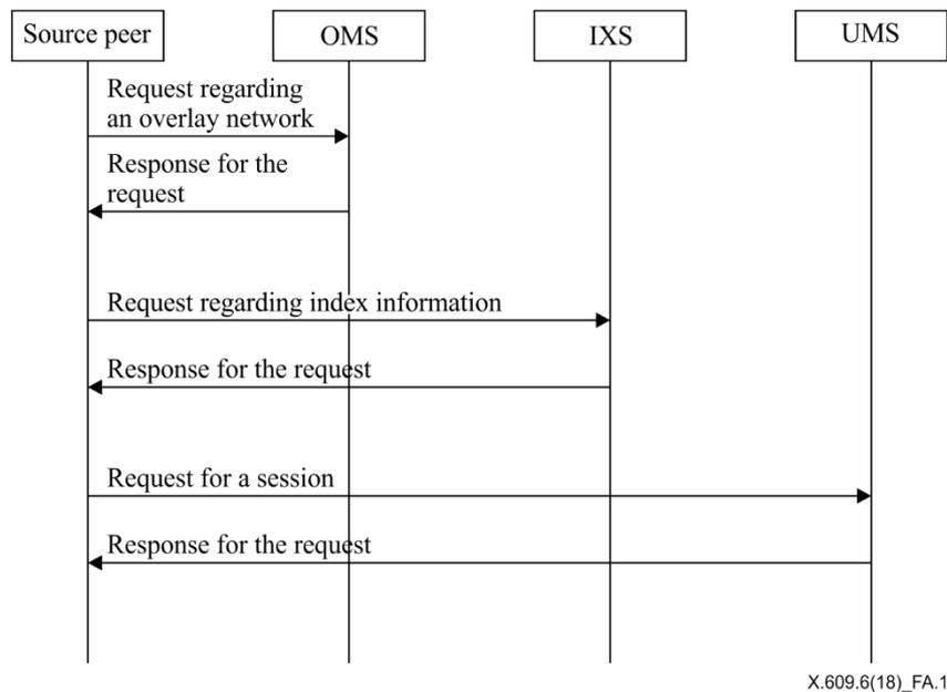
**Figure A.1 – Source-side procedure of content distribution**
