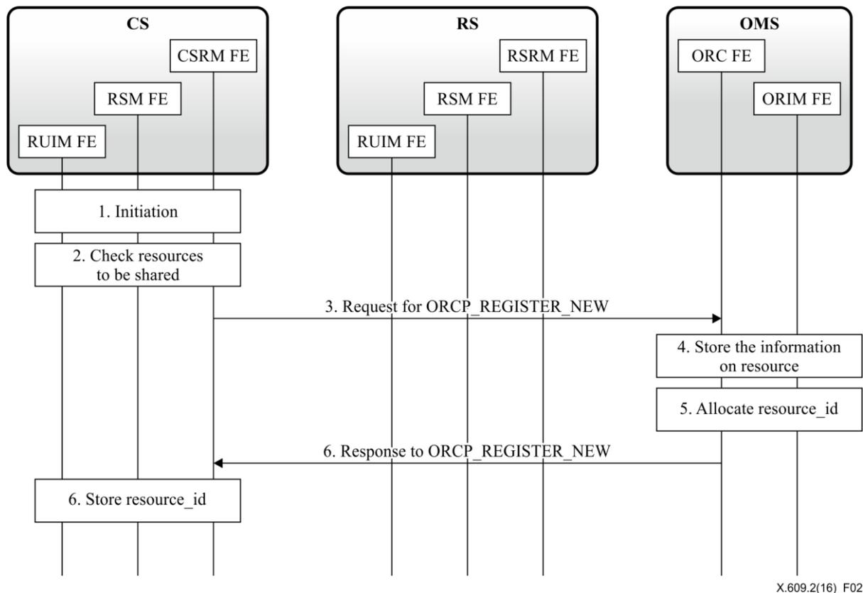
**Figure 2 – Flow for registration by CS/RS**
