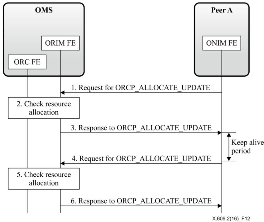
**Figure 12 – Flow for refreshing resource allocation**
