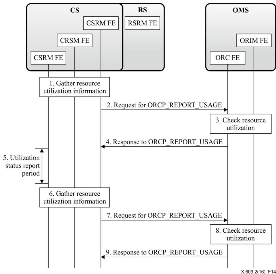
**Figure 14 – Flow for CS/RS resource utilization report**
