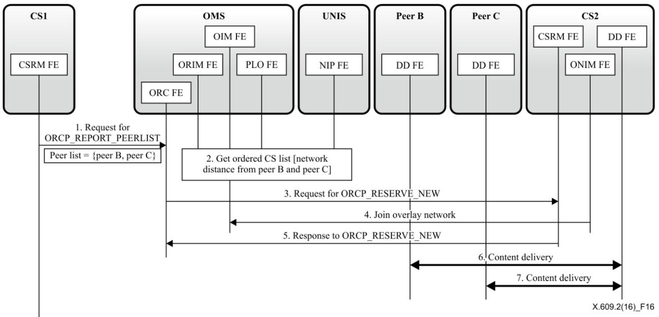
**Figure 16 – Flow for selecting a new CS to be added to an overlay network**
