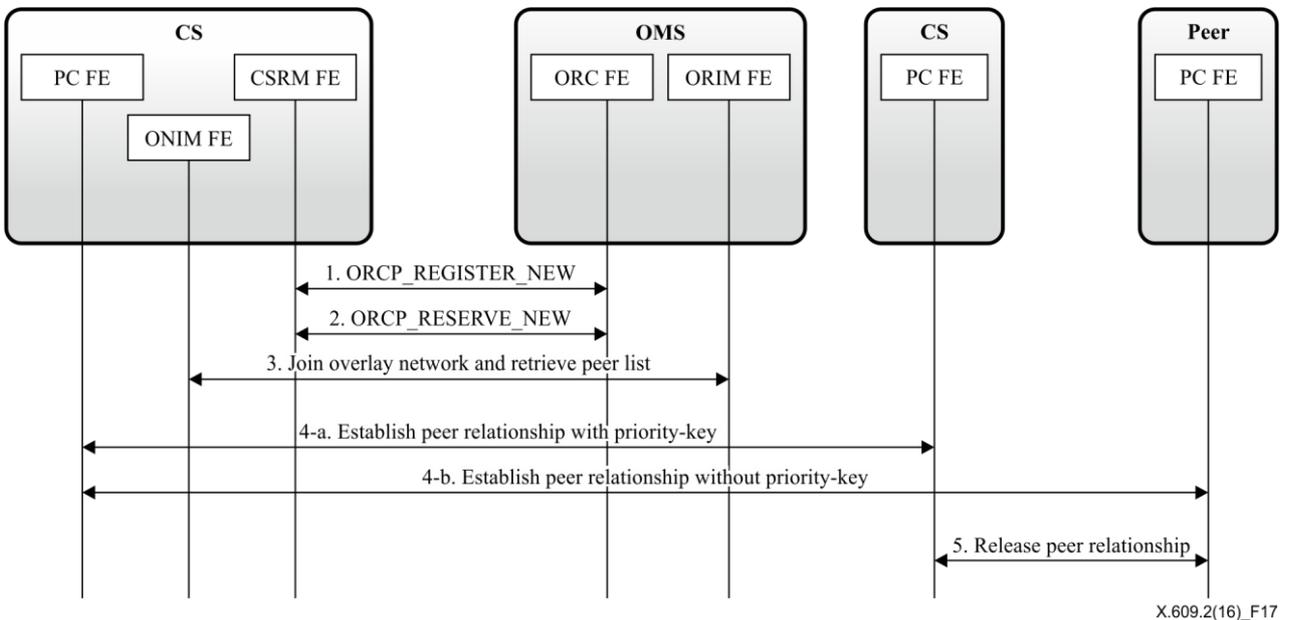
**Figure 17 – Flow for prioritization of virtual peers of a CS**
