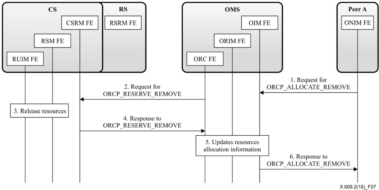
**Figure 7 – Flow for release of overlay resources**
