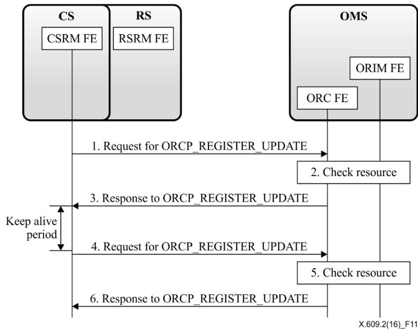
**Figure 11 – Flow for refreshing CS/RS registration**
