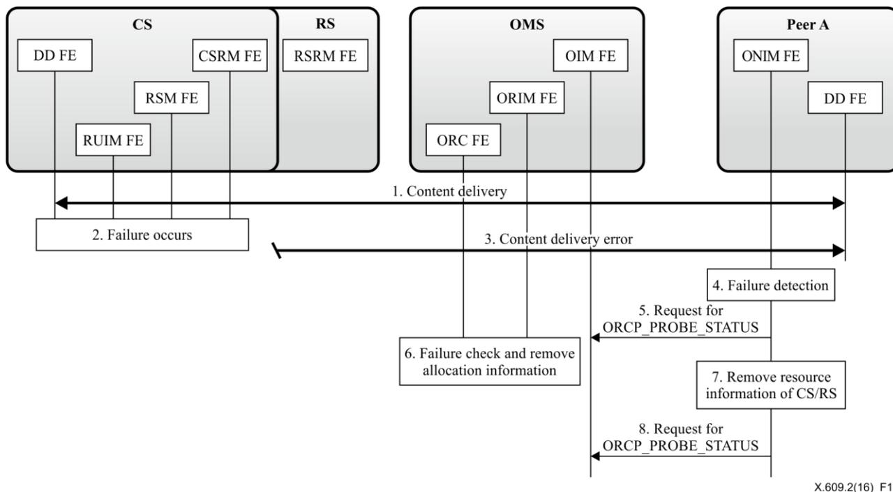
**Figure 10 – Flow for failure recovery on CS/RS error**
