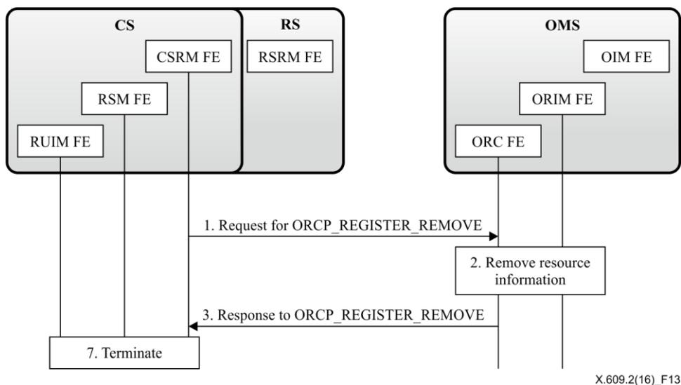
**Figure 13 – Flow for deregistration of CS/RS**
