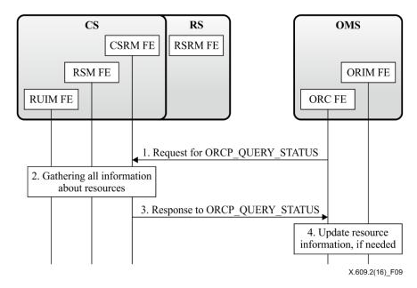
Figure 9 – Flow for probing full resource allocation status
