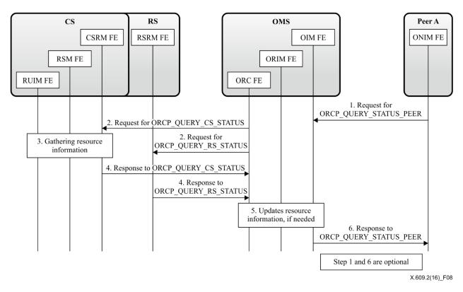
Figure 8 – Flow for peer probing resource allocation status
