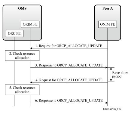
**Figure 12 – Flow for refreshing resource allocation**
