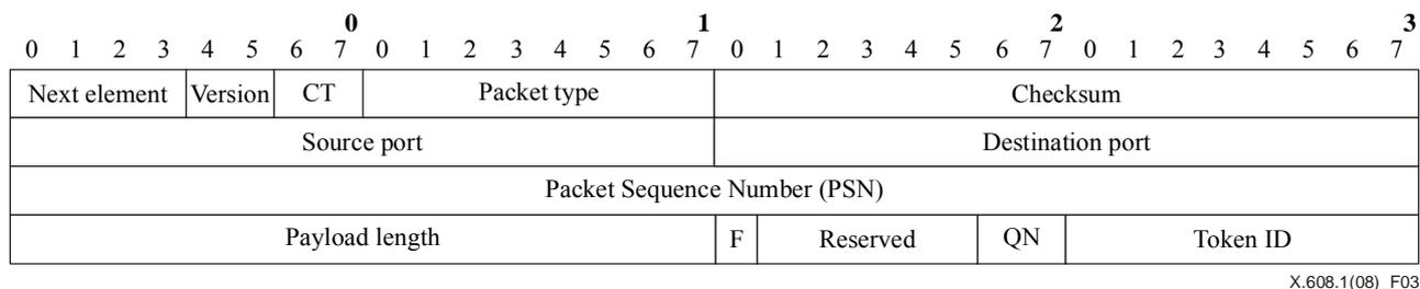
**Figure 3 – Base header in ECTP-5**
