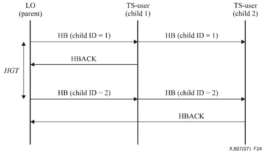
**Figure 24 – Tree maintenance using HB and HBACK packets**
