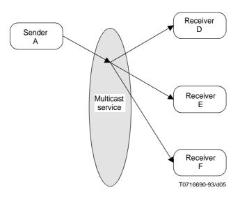
FIGURE 5/X.6 One-way data transfer (simple case)
