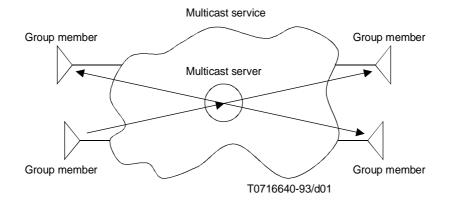
FIGURE 1/X.6 Multicast service model
