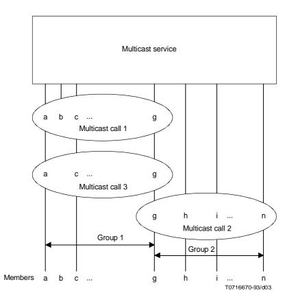
FIGURE 3/X.6 Examples of call configurations
