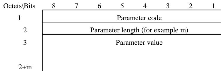
**Figure 5 – Structure of parameter within variable part**
