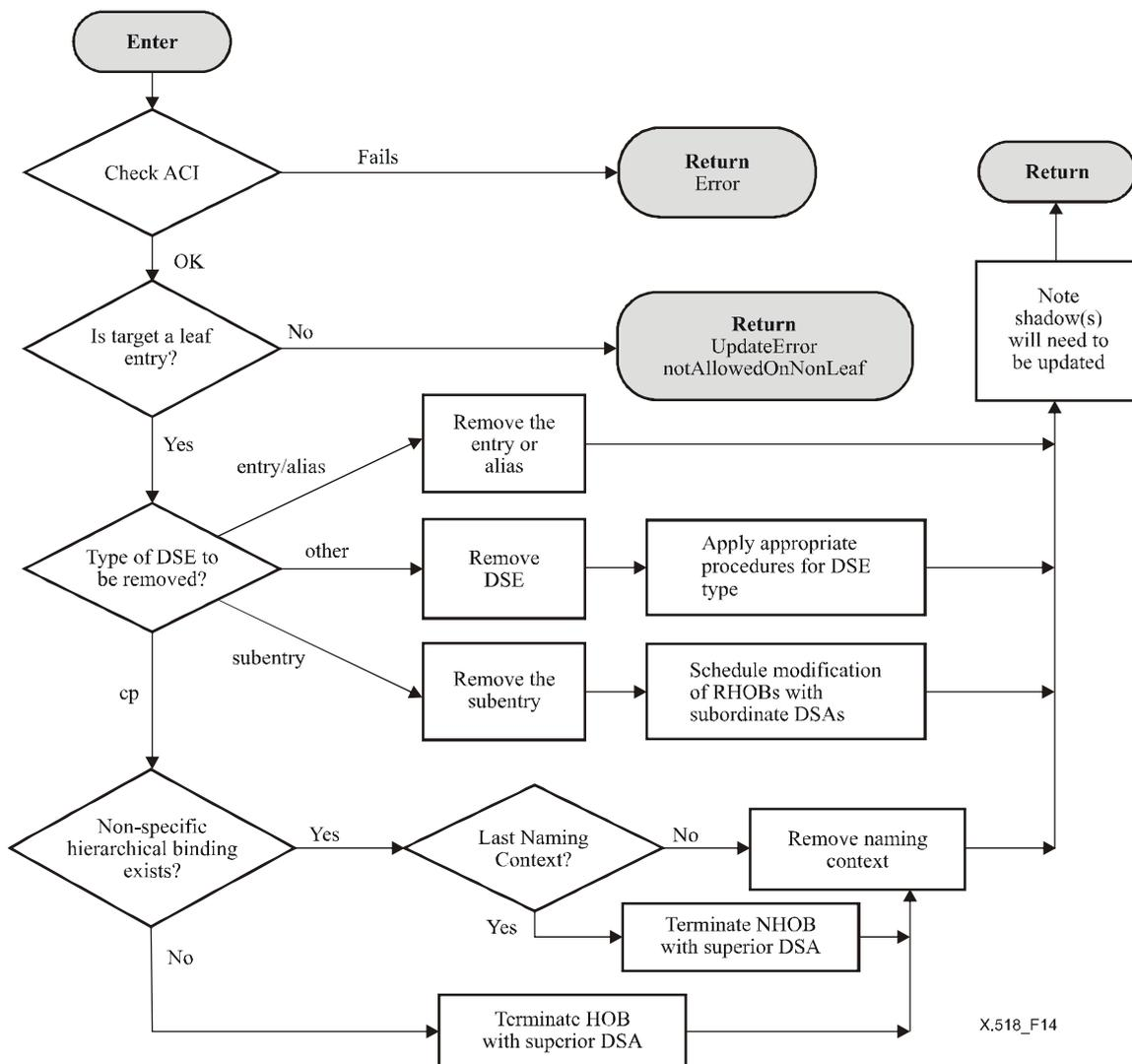
Figure 14 – DAP Remove Entry procedure
