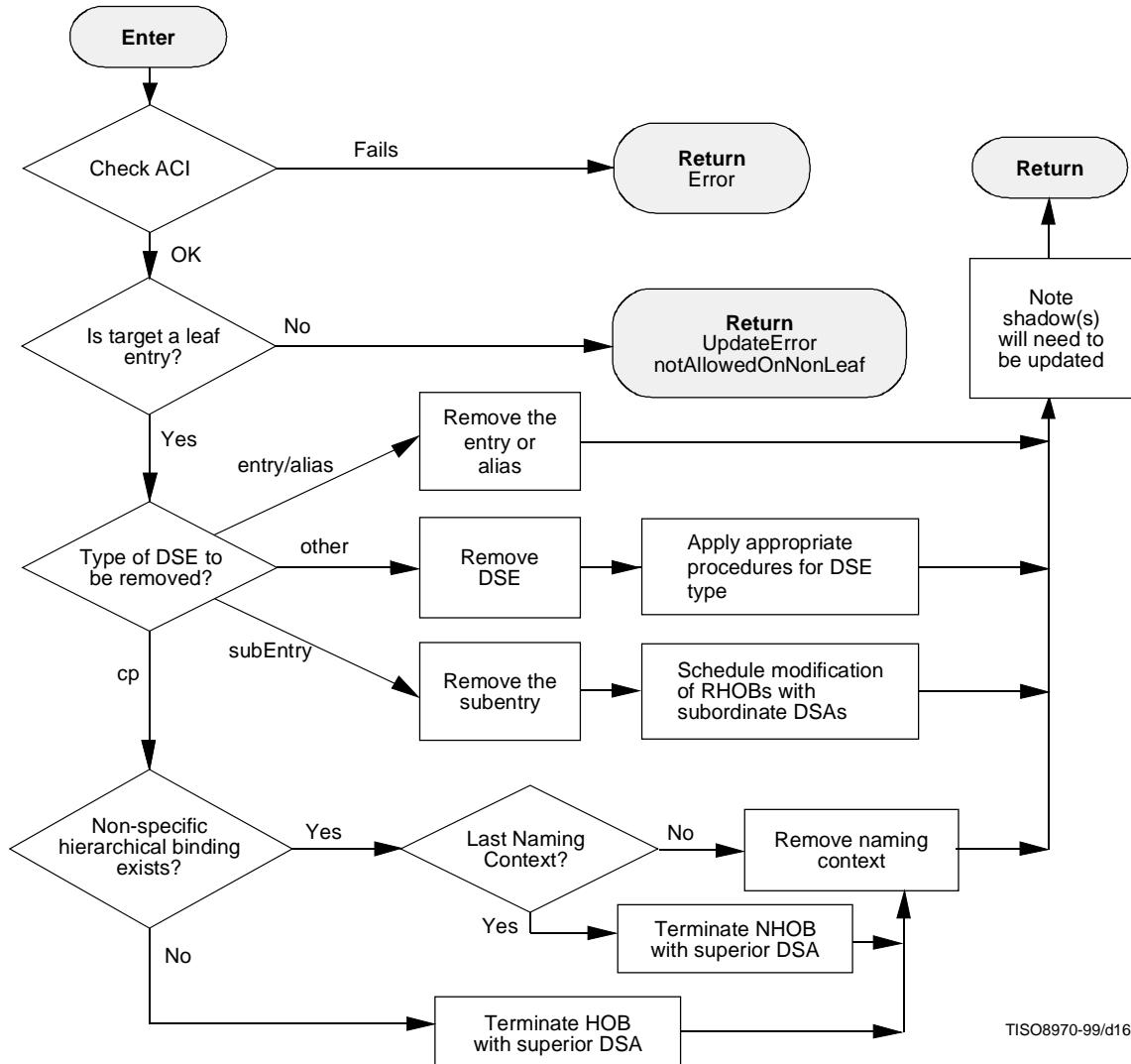
**Figure 14 – Remove Entry procedure**
