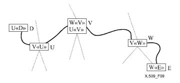
Figure 9 – Non-hierarchical certification path – An example
