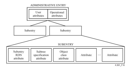
Figure 10 – Structure of a Subentry
