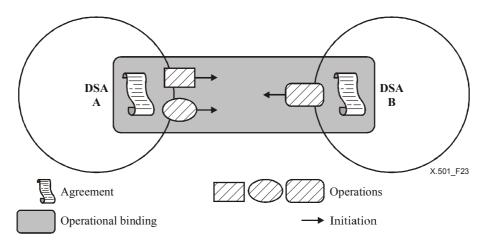
Figure 23 – An operational binding
