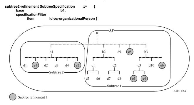
Figure K.2 – Subtree specification example
