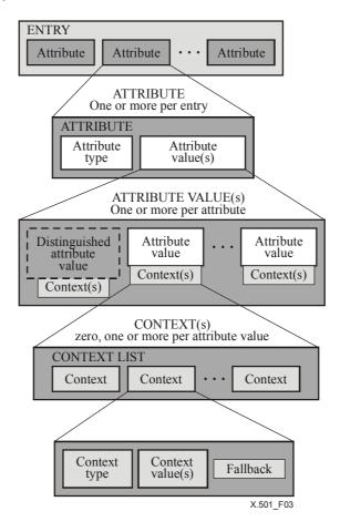
Figure 3 – Structure of an entry
