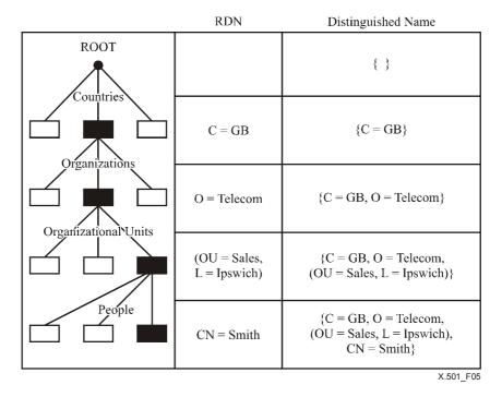
Figure 5 – Determination of distinguished names
