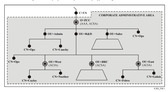
Figure M.1 – DIT branch for the Z Computer Corporation (ZCC)
