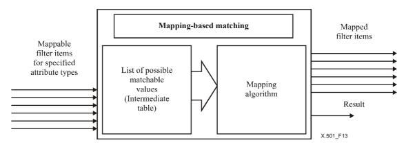
Figure 13 – Mapping-based matching
