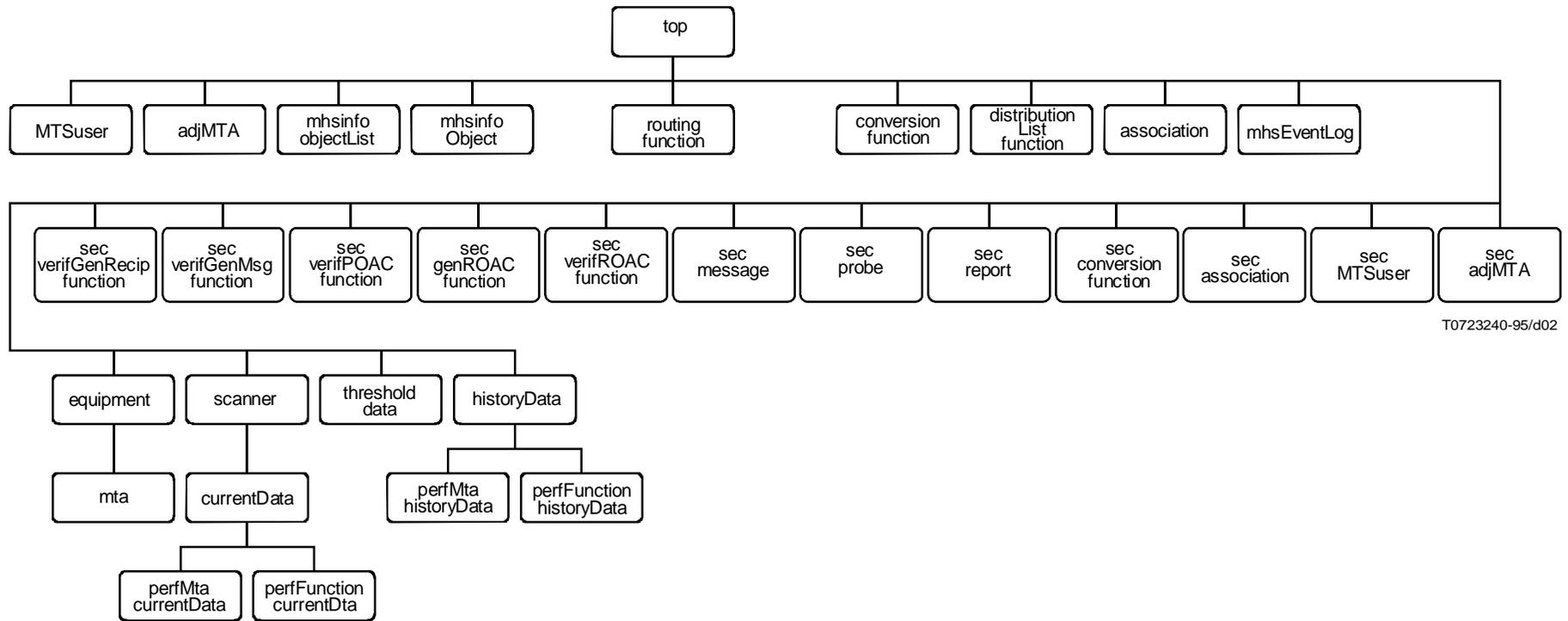
Figure 2 – Inheritance tree for MTA management
