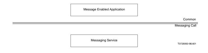
Figure 1/X.446 – Positioning of the Common Messaging Call API
