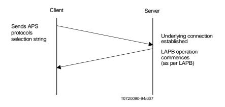
FIGURE 7/X.445 Normal LAPB data link set-up (no errors)
