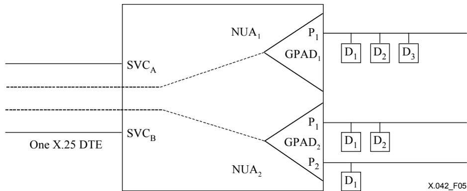
**Figure 5/X.42 – PAD expanded configuration – Two GPAD instances**
