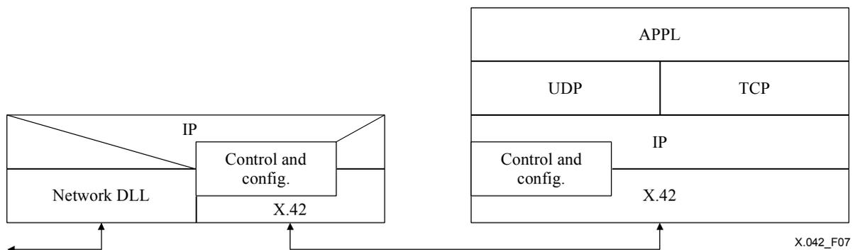
**Figure 7/X.42 – Internal organization of GPAD terminal IP-enabled;
