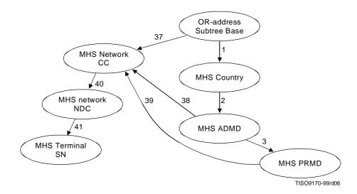
Figure E.1 – OR-address subtree schema for MHS Network Address
