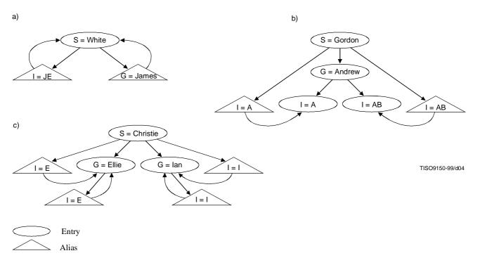
NOTE 1 – Example a illustrates the case where a particular Surname is unique in this OR-address-subtree. Alias entries are created corresponding to the optional Initials and Given Name elements.
