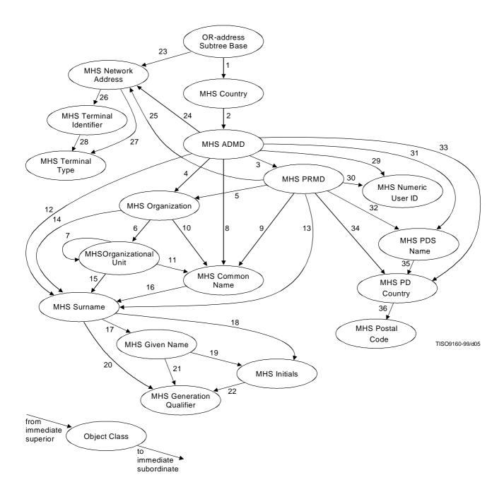
Figure D.1 – OR-address subtree structure
