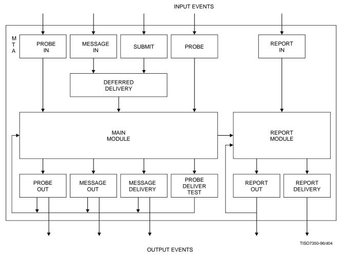
Figure 6 - Relationship of internal and external modules
