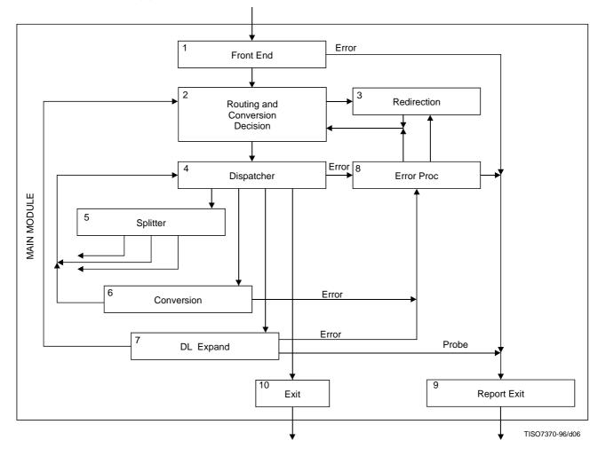
NOTE – Numbers in this figure refer to the numbered steps in the control procedures logic (see 14.3.1.4).
