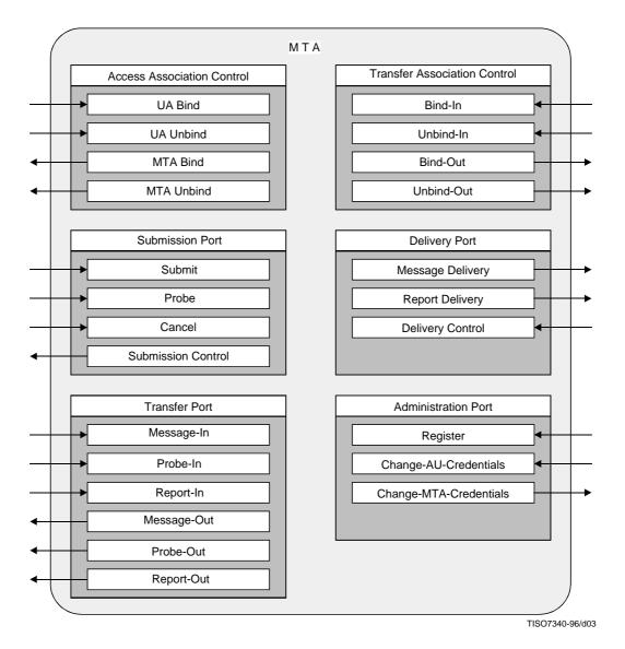
Figure 5 – Ports and modules of an MTA
