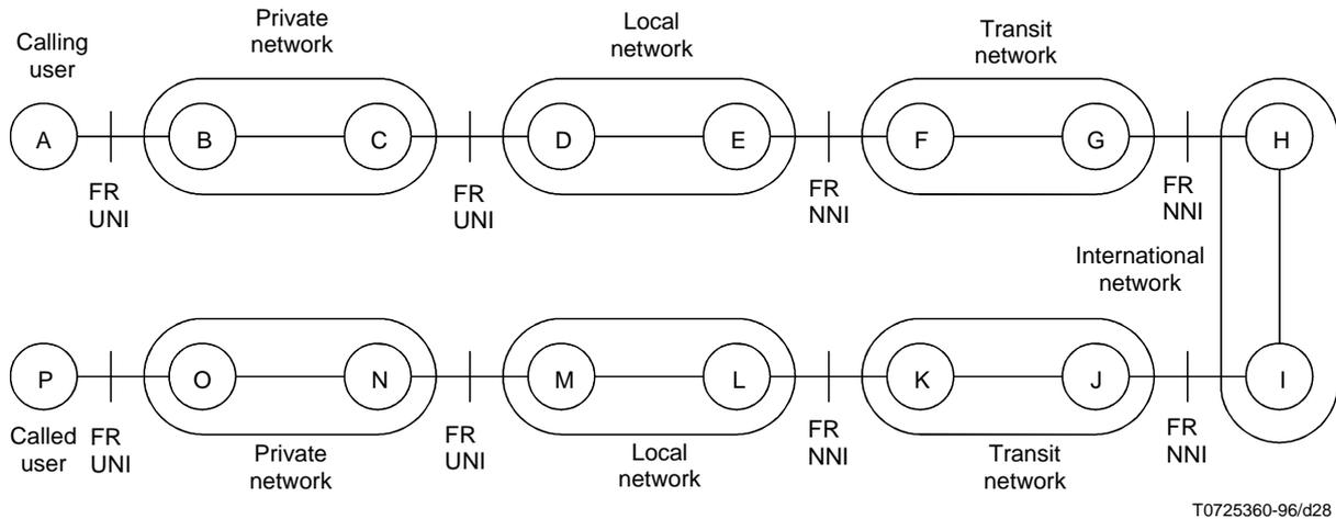
NOTE – The interface A-B, C-D, M-N and O-P is assumed to be Frame relay UNI.
