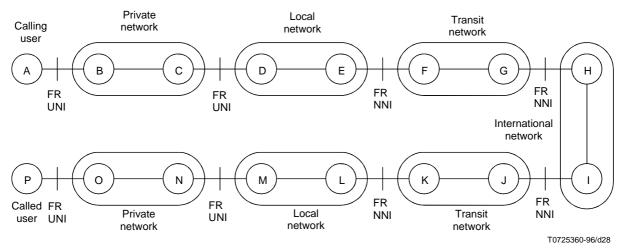
NOTE - The interface A-B, C-D, M-N and O-P is assumed to be Frame relay UNI.
